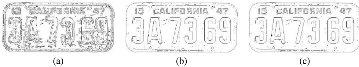
Figure 9. Edges detected by the (a) Canny, (b) Sobel, and (c) Prewitt edge detection methods on the test image.
