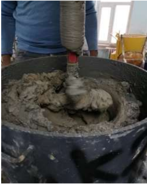
Figure 5. Creation of a deep mixing column in the large-scale experimental setup
