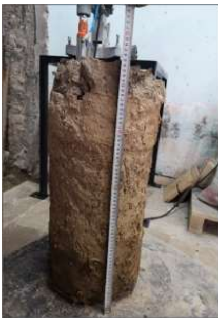
Figure 6. Large-scale deep mixing columns
