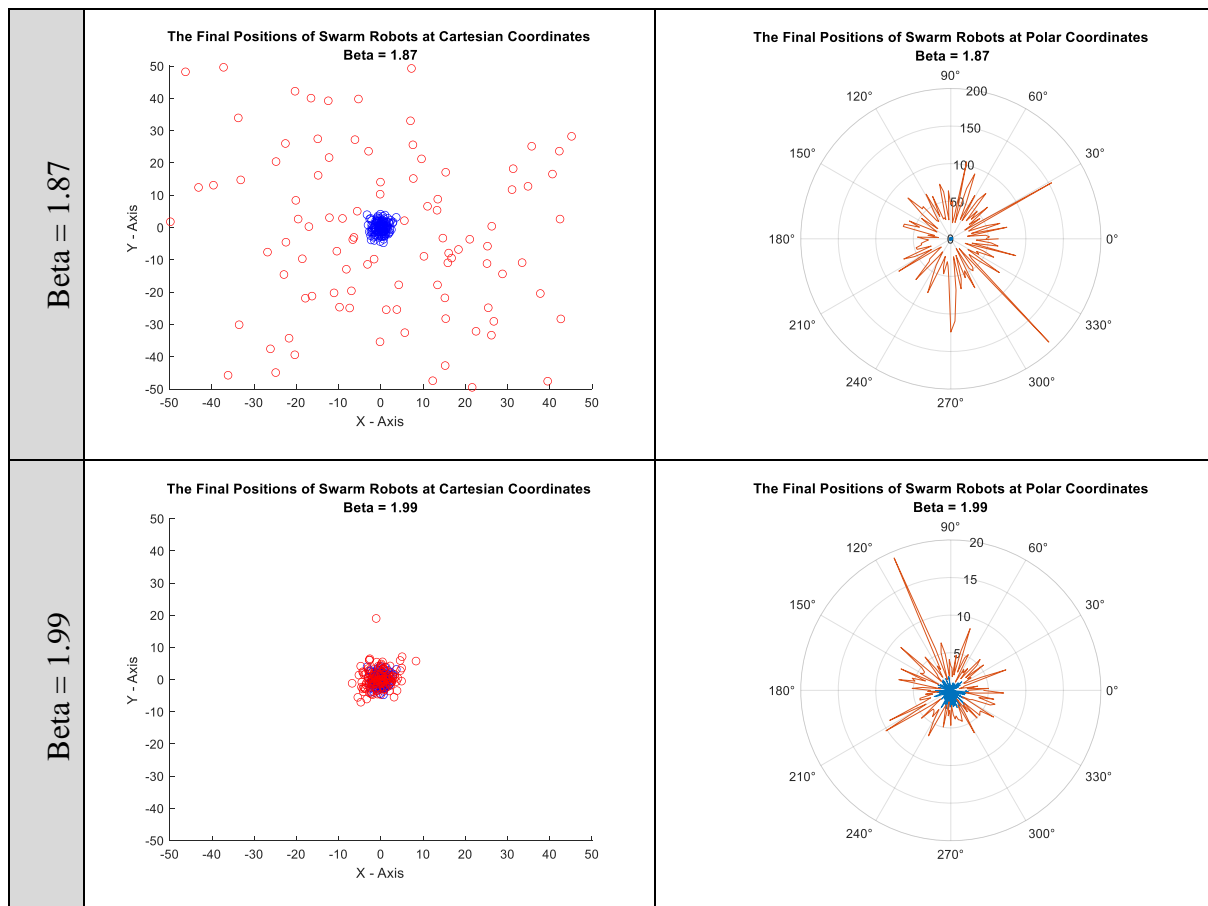
Figure 1. The Final Position Results of Swarm Robot Simulations Based on Different Values of the Beta Parameter of the Levy Walk Algorithm
